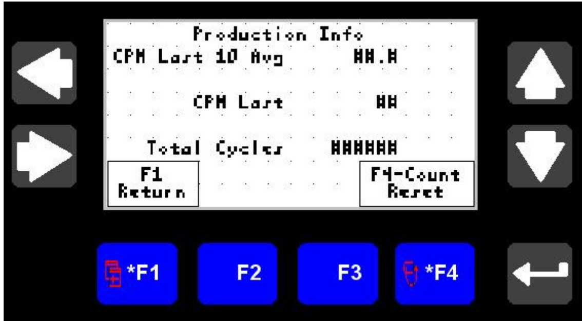
Figure 7 - HMI Control Panel – Product Information Screen
