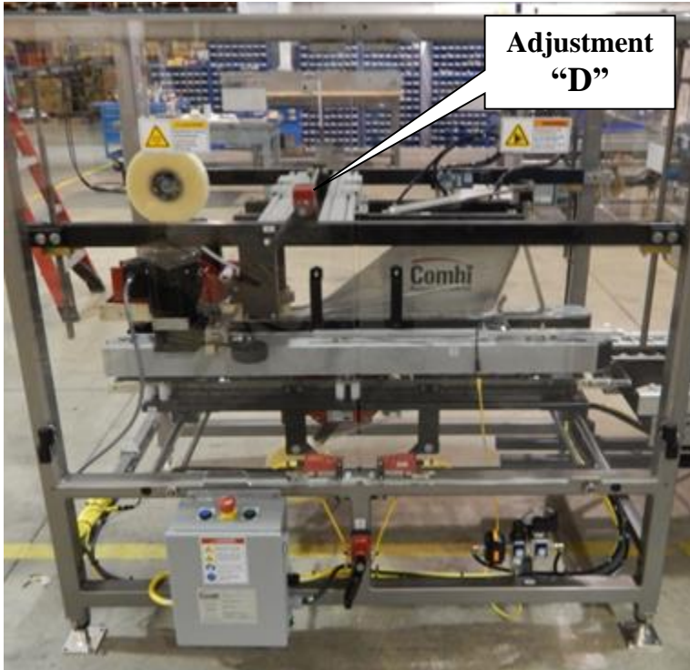
Upper Tape Head / Plow Assembly Adjustment Location
