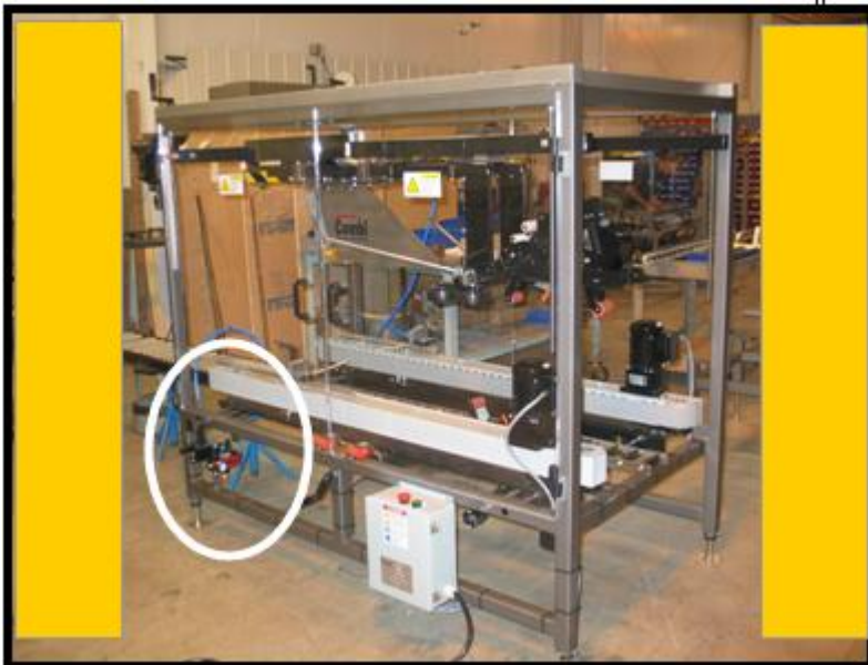
Figure 4C - Location of Main Air on Right Hand Execution Stand Alone Machine.
