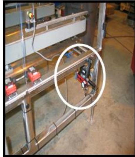
Figure 4B - Location of Main Air on Left Hand Execution Stand Alone Machine.
