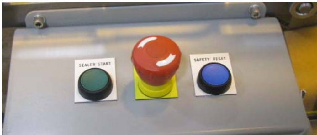
Figure B2 - Located on upper frame or on electrical box. Shown here on electrical box.
