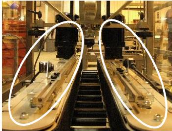
Figure 7 - Belt Drive and Motors.
