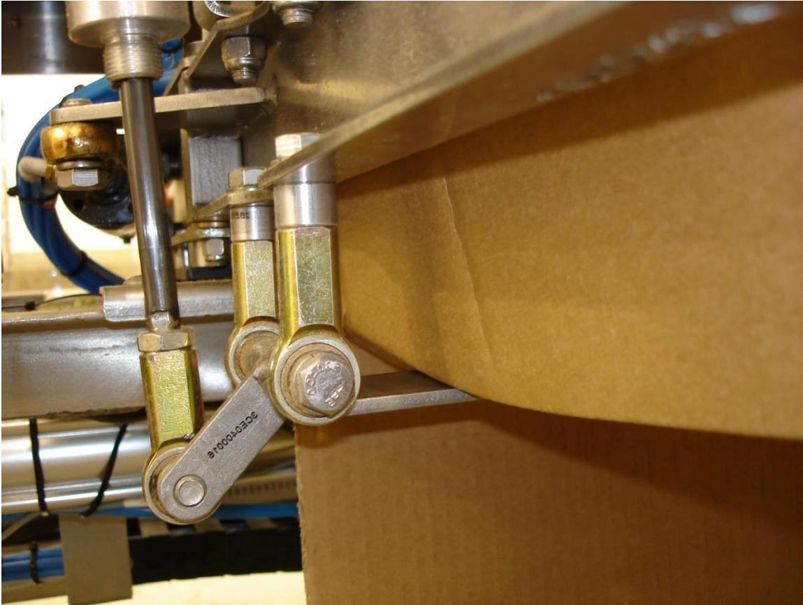
Incorrect Case to Flap Kicker Placement
