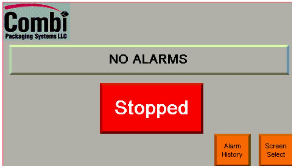
The Main screen shows if machine is running or stopped and allows the operator to navigate to other screens.
