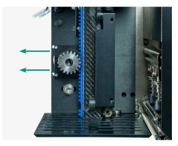
5. Check that the gear is securely tightened onto the motor shaft. The gear is held securely in place with set screws located on the collar of the gear.
