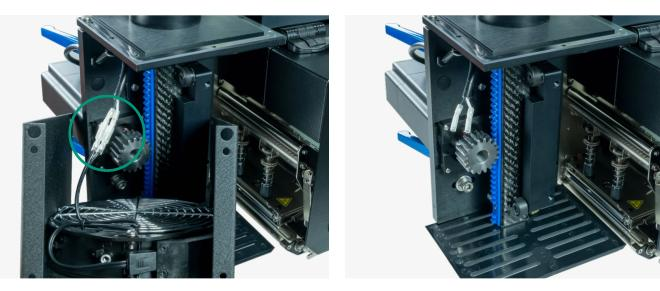
3. Loosen the four (4)  $1/4-20 \times 1/4''$  mounting bolts on the applicator motor.
