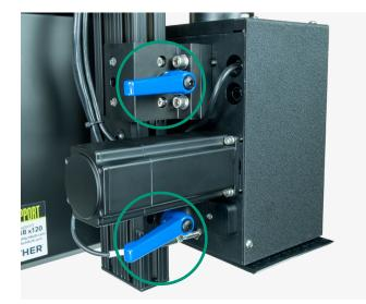
13. Adjust the vertical position of the tamp head so that the print engine peel bar splits the bevel on the tamp head. Note: This well require adjusting the fixed mounting bolt that the slide assembly rests on. You should position the surface of the tamp head approximately 1/16" below the position where the labels feed out.
