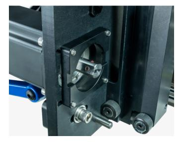
Using even pressure on the motor, push the applicator drive motor back towards the applicator rack.
