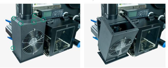
2. Remove fan shroud and disconnect the power wires from the fan.
