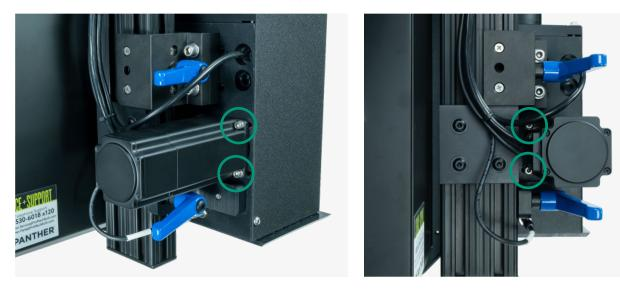
4. Slide the applicator motor and gear away from the applicator rack.
