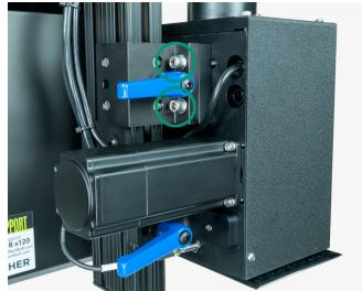
12. Loosen the vertical adjustment lock handles, located on the back of the Predator main plate.
