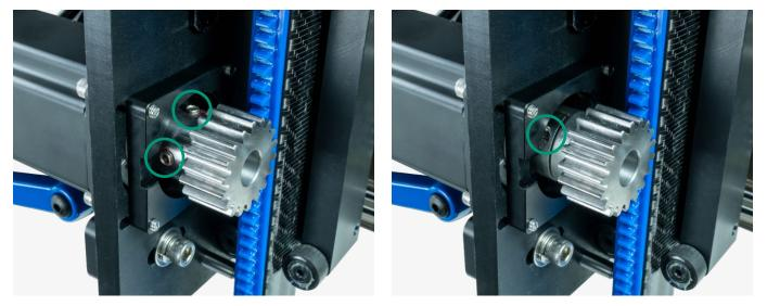
These set screws should be tightened onto the center of these flat spots. Thread lock may be used to prevent these set screws from coming loose over time. The gear should be positioned such that the teeth of the rack are centered on the teeth of the gears. **Note: The motor shaft has two (2) keyed flat spots.**
