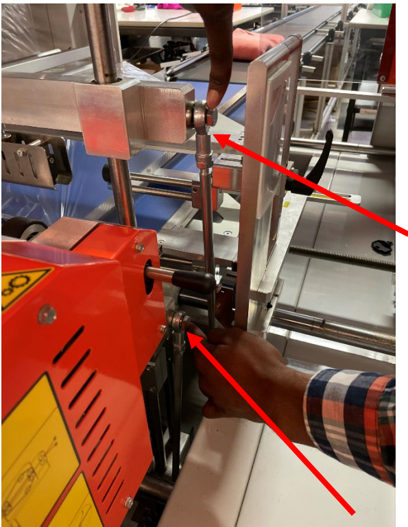
Figure 17. Connecting rod shafts requiring monthly grease application.
