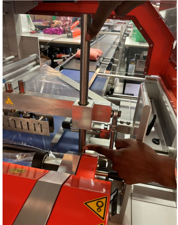
Figure 16. Vertical seal bar shaft requiring monthly grease application.
