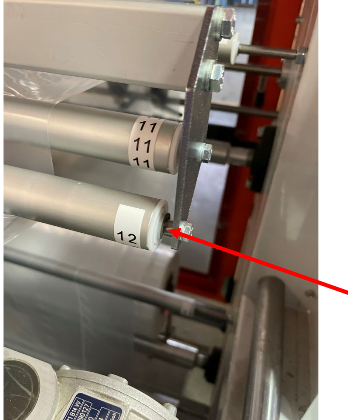
Figure 20. Retaining ring monthly visual inspection.
