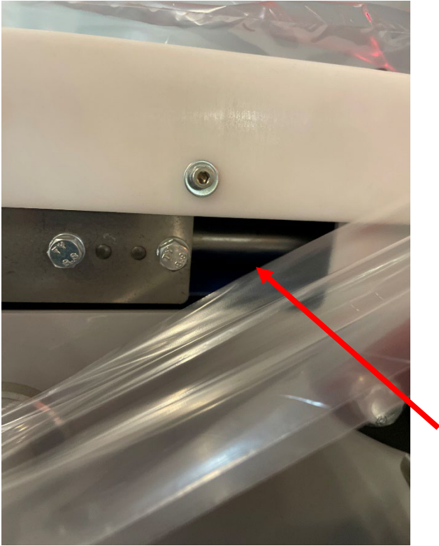
Figure 15. Indexing conveyor shaft requiring monthly grease application.
