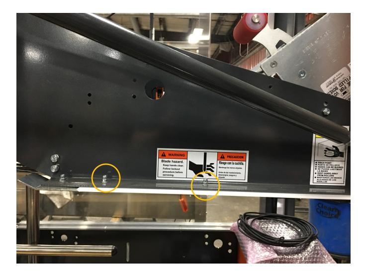
Remove these two dome nuts, screws and washers marked above on both sides of the head.
