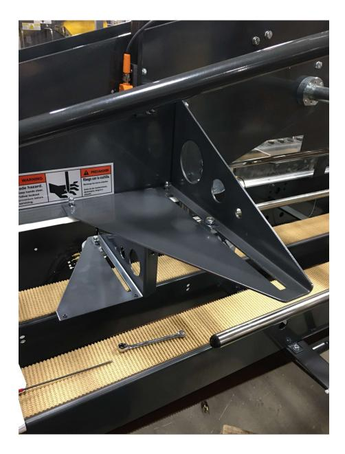
Place the squeezer bracket for that side of the head with the horizontal piece facing the exit of the machine. Replace the screws with the 16mm ones provided and tighten them only enough to hold the bracket in place.
