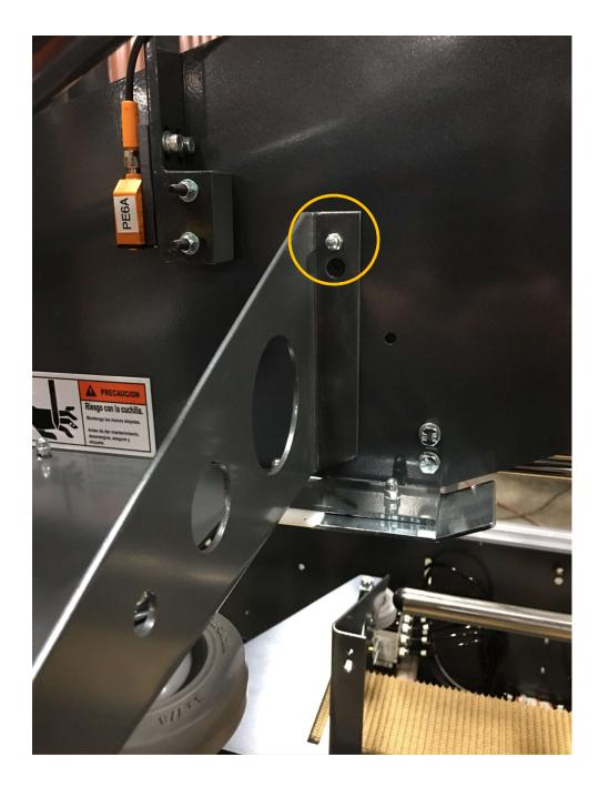
Now all fasteners can be tightened and the wheels can be adjusted to the proper width to close the box.
